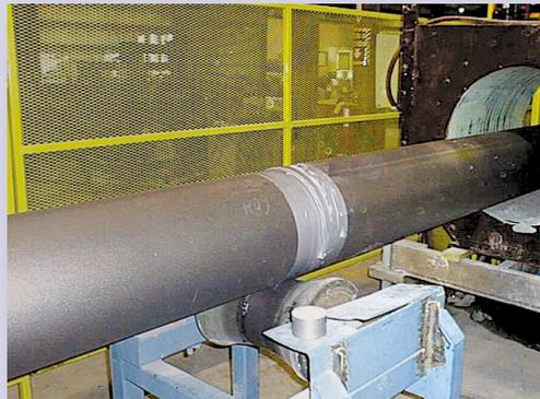
Among the many applications, seal and join a butt splice for pipe ends in a coating process.
